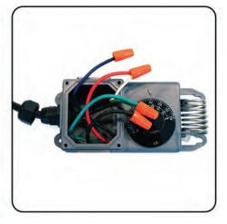
Switch the blue and red wires. The white and red wires should now be joined and the blue wire should be capped alone. Push the wires back into the box. Replace the panel with the 4 screws and you are ready to control your heater.
