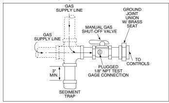
• Manual shut-off valve is in "off" position when perpendicular to pipe.
