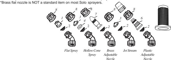
No-drip-check valve replaces # 2 on heavy-duty (HD) models along with O-rings 0062106 and 0062115.
