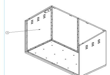
Position LH side panel 5 next the the LH rear panel 4 and base panel 2 ensure all holes are aligned along the base and side then screw together.
