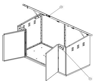
Position the grab handle (16) on the front of the lid (12) in the centre ensure holes are aligned and screw into place using set screws (18). Check the lid closes flush before fitting the Locking shrouds (17) these are fitted one on each infill panel (6). Align the holes and screw into place again using countersunk screws 21. Ensure the locking holes all align before attaching the padlock, incorrect alignment could damage the lock.
