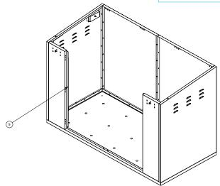
Door catch (9) can now be fitted, position on the inside of the unit slotting into the Infill panel 6 positioned on the left hand side. This will be slightly overhanging to catch the door. Align the holes with the Infill panel 6 and screw together.
