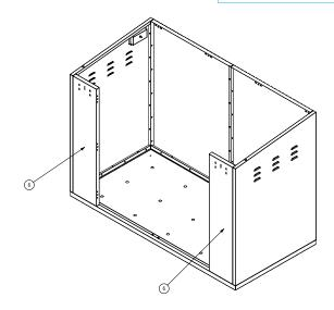
Position an Infill panel 6 next to the LH Side panel 5 ensure all holes are aligned along the base and side then screw together.
