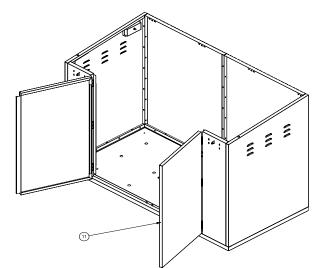
Support the doors at all times whilst fitting the counter sunk screws (21) to ensure correct alignment, always use a hand held screwdriver.
