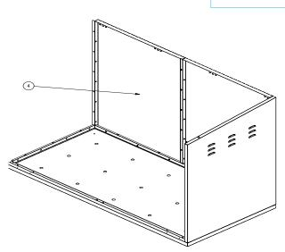
Position LH (left hand) rear panel 4 next to RH rear panel 1 and base panel 2 ensure all holes are aligned along the base and side then screw together.
