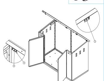
Lift the Lid (12) on to the unit, position Hinge fixing bracket (13) on to the back of the unit pushing the screws through the holes of the hinge attached to the Lid and the holes of the Back panel, then position Hinge support bracket (14) on the inside of the unit over the screws, use Nuts (20) to secure the screws.
