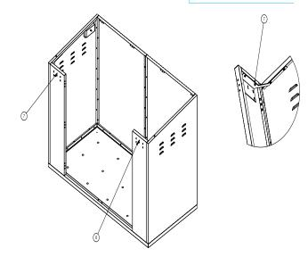
Position the LH Support bracket 7 into the top corner connecting the Infill panel 6 positioned on the left and the LH Side panel 5, ensure the holes are aligned and screw together.
