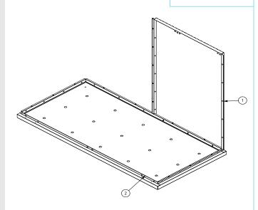
Position RH (right hand) rear panel 1 against the base panel 2 ensure all holes are aligned.
