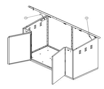
The Gas damper (15) can now be fitted, the thinner end of the gas damper should be positioned and attached to the LH side panel 5 and the thicker end of the gas damper should be attached to the lid (12). Repeat with the second gas damper (15) attaching to the RH side panel (3).
