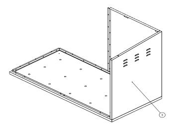
Position RH side panel 3 next to RH rear panel 1 and base panel 2 ensure all holes are aligned along the base and side then screw together.
