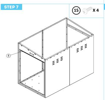
Attach the Fascia panel (8) across the front of the unit as pictured. Screw into both the Front side panels (6) and (7).
