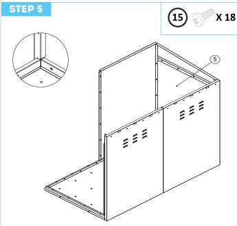
Position Back panel (5) into the groove on the base panel (1), between the side panels (2) and (3), and under the Back Fascia panel (4). Ensure the holes along all four sides are aligned and screw together, tighten the screws for the Back Fascia panel.
