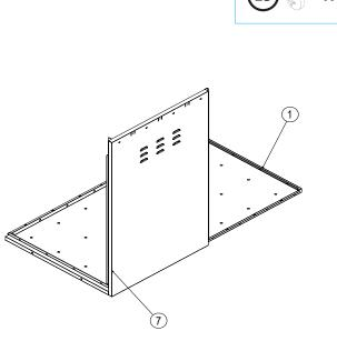
Position Front RH (right hand) side panel 7 into the groove on the Base panel 1 ensuring the holes are aligned.
