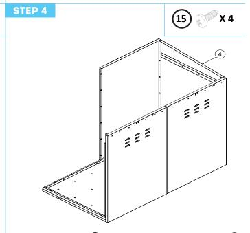
Position Back Fascia panel 4 between the two Rear side panels 2 and 3 at the top of the unit. Ensure the holes are aligned and loosely screw together, creating a gap for the back panel.
