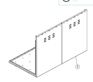
Position Rear RH (right hand) side panel 3 into the groove on the base panel 1 and the already fixed Front RH (right hand) side panel 7, ensure the holes are aligned and screw together.
