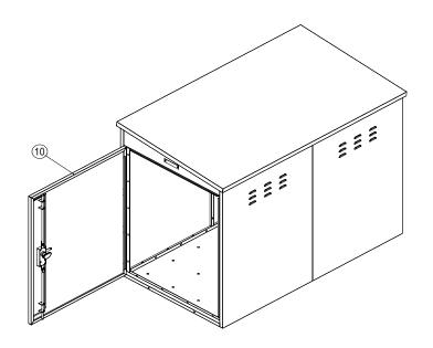
Support the door at all times whilst fitting the counter sunk screws 16 to ensure correct alignment, always use a hand held screwdriver. Position the Door 10 so that the hinges are aligned with the fixing holes, screw together.
