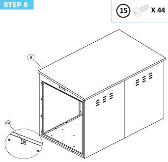
Lift the Roof panel 9 onto the unit, covering the other panels and fascia panels. Screw into place using the single screw holes. Fit the Roof security brackets 14 in the pair of slots on the top of each of the panels, each bracket is fitted with a single screw.
