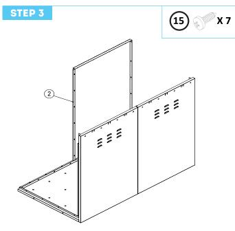
Position Rear LH (left Hand) side panel 2 into the groove on base panel 1 and opposite the already fixed Rear RH side panel 3 Ensure the holes are aligned and screw together.
