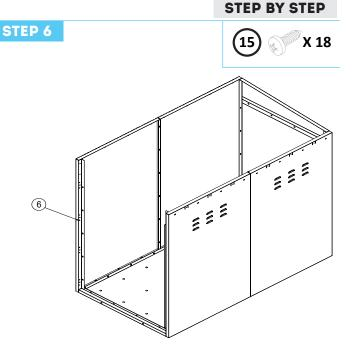
Position Front LH side panel 6 into the groove on the base panel 1 and Rear LH side panel 2. Ensure the holes are aligned and screw together down the full length of the vertical joint and across the base.
