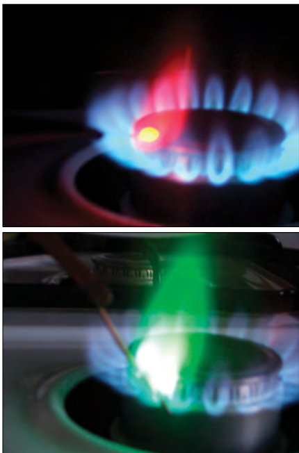
Figure 1.14. Lithium (top) and copper flame tests.
