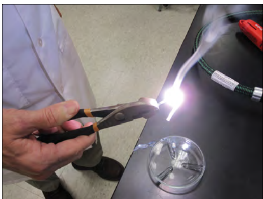
Figure 10.18. Burning magnesium, which lights with a butane lighter, but not with a match.
