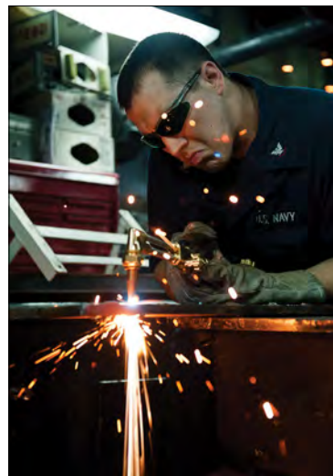
Figure 10.14. The flame from an oxyacetylene torch cuts right through steel plate.
