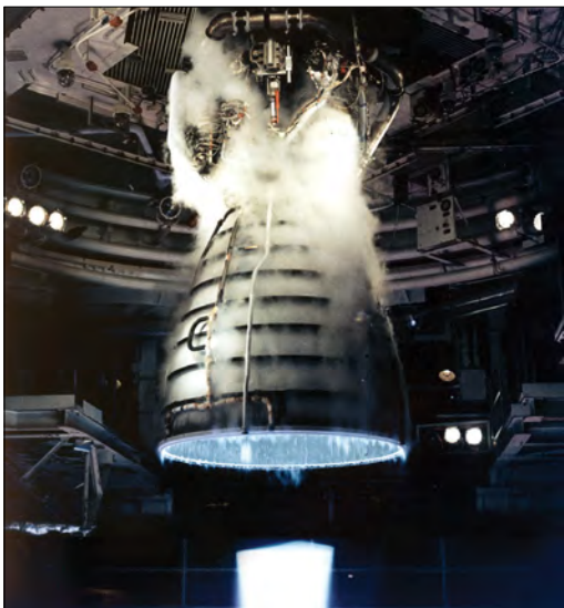
Figure 10.1. The chemical reaction between liquid hydrogen and liquid oxygen is the energy source used by the Space Shuttle main engine. The white formation under the engine at the bottom is water vapor that has condensed to liquid droplets, allowing the water vapor to become visible.
