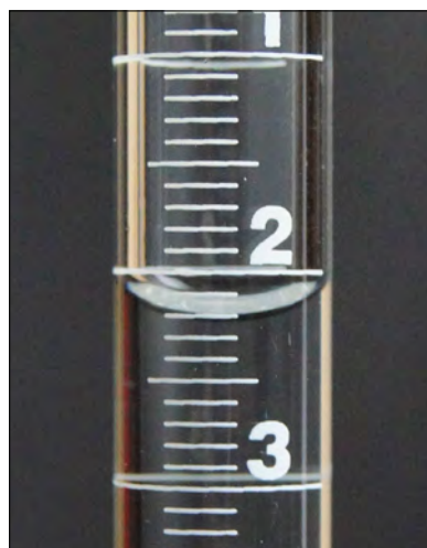
Figure 2.4. Reading the significant digits on a buret.
