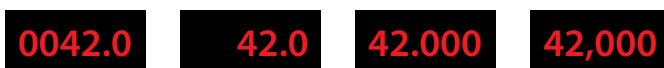
Figure 2.2. With digital instruments, all digits are significant except leading zeros. Thus, the numbers of significant digits in these readings are, from left to right, three, three, five, and five.
