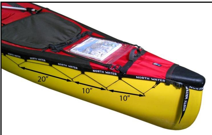
Lay your spray deck out over your canoe. The bow end of the deck (underside) is marked with a label indicating brand and model of canoe for which the deck was made. Check the direction of the cockpit hook and loop closures; they should face forward. The bow and stern straps should be placed under the bow and stern end caps. Use the adjustable tensioning end straps to snug it up and centre it fore and aft. You do not want to put a lot of tension on the deck with this strap.
