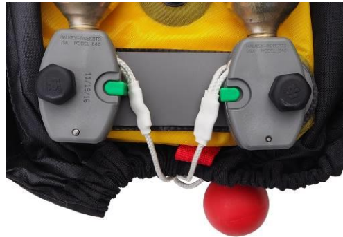
B. Place the folded Rescue Float into the pouch with the cylinders facing up.
