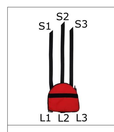
1. Slide **S1** through top webbing closest to zipper, **S2** through top webbing on other side of belt loop and **S3** through top webbing farthest to the right. **S2** and **S3** are over top of the Quick Release Chest Harness.
