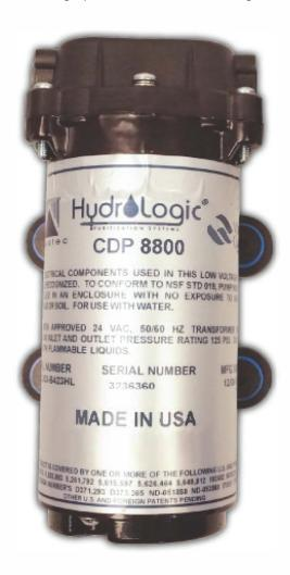
Note: The Stealth-RO operates at 40-80 PSI. There is an adjustable allen screw on the front if the pump to dial in the pressure if needed. Ideal PSI is 65. You'll need a 1.5 millimeter allen wrench.
