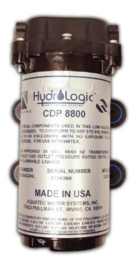
Note: The Stealth RO operates at 40-80 PSI. There is an adjustable allen screw on the front if the pump to dial in the pressure if needed. Ideal PSI is 70. You'll need a 1.5 millimeter allen wrench.
