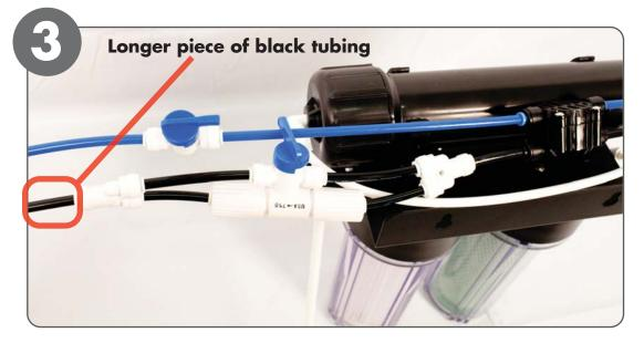
4) To "power flush" the membrane(s) simply turn the ball valve (on the blue product line) to the off position and turn the ball valve on the black waste water line to the open position (parallel to the black waste water line). Flush membrane(s) for 3-5 minutes after each use or at least once a week. This will extend the life of your membrane(s). Once finished flushing turn both the ball valve handles back to their position displayed in step 3 for normal operation.
