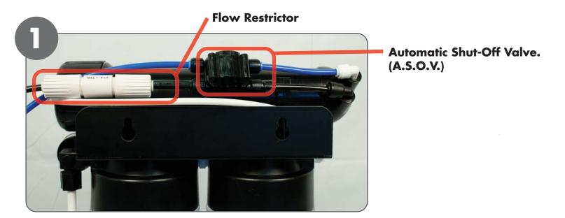
2) Insert flow restrictor into flush kit by pushing the open ends of the tubing into the quick connect fittings. Make sure the arrow is pointing in the direction of water flow (away from the RO unit)
