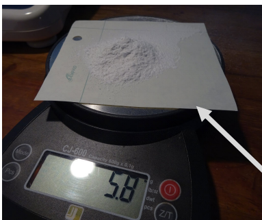
This filter was loaded with 5.8g of dust.
