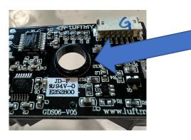
You can use a clean cotton swab (Q-Tip) inserted into the ring and gently wiping around in a circular motion, then blow air through the ring to ensure it's clean.
