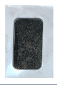
Tip: In most cases, blowing forced air into this chamber will clear any debris that might cause inaccurate readings. You can do this with compressed air, a hairdryer or deep dry breaths.
