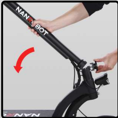
③ Lower the handlebar.
