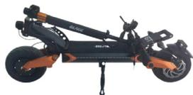
2. Lift the handle post into a vertical position. And fasten both quick release buckles.
