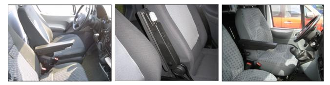
Armrest model ML385 is recommended for light and heavy trucks. Choose from different materials and colours on the top-cover, such as PUR, Textile, Vinyl or Leather. The armrest-base material is Polyamide. See our variety of standard armrest on the next page.
