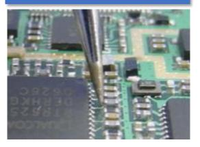
Set 0603 as an example; very fine tip end makes it easy to solder a tiny chip.
