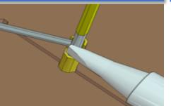
Put the cut surface to the lead and terminal at one time to heat them. Feed solder to form smooth fillets. Note: Get rid of gold plating of terminal and pre-tin lead wire. It makes solder spread over the terminal easily and prevents soldering defect.
