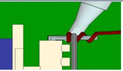
Put the cut surface to the coil and terminal at one time to heat them. Feed solder.
