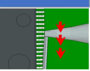
Put the tip end to the leads and drag it slowly. Note: Apply flux to leads and land pads before soldering. It prevents the troubles such as solder bridge.
