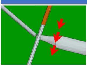
Put the cut surface to the lead and drag the tip slowly while feeding solder.
