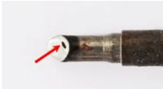
Corrosion of Soldering Tip
