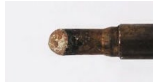
Oxidation of Soldering Tip
