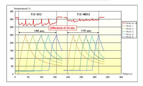
The high heat capacity reduces the time taken to solder each point, overall causing a significant decrease which increases efficiency in the long run.
