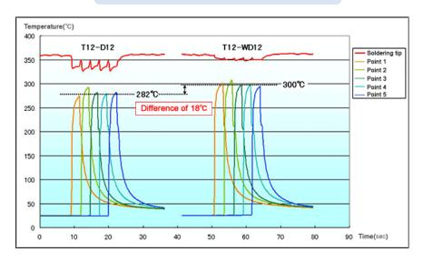
With the heavy duty tip's increased heat capacity, the temperature of the workpiece is increased, allowing the solder to melt easily.
