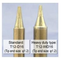
Heavy duty soldering tips are derived from the shapes B, D and I with a thicker radius along its body to increase heat storage. This makes it best suited for work requiring high heat capacity.
