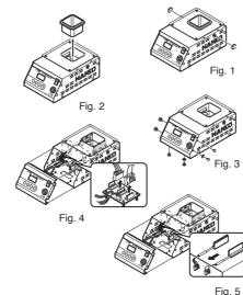
1. Using the hexagon wrench (provided with the HAKKO FX-301B) to loosen the screws on both sides of the unit.
