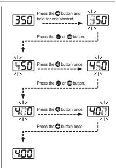
For the  $50 \times 50$  square pot, the setting range of temperatures is between 200 - 450°C/400 - 840°F. For the  $75 \times 75$  square pot, the setting range of temperatures is between 200 - 380°C/400 - 720°F.
