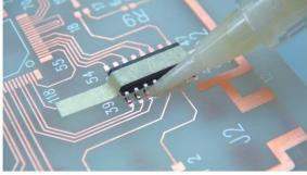
Simply push the shaft for a generous coating of flux
