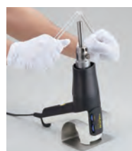
Curving plastic material Use of nozzle holder and single nozzle
