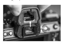
2. Align the groove on the EP-NZP with the rails on the camera's viewfinder.
