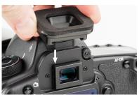
3. Firmly slide the EP-N down on the viewfinder rails until fully seated.
