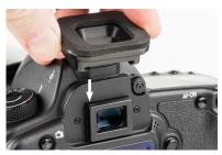
3. Firmly slide the EP-15 down on the viewfinder rails until fully seated.
