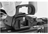
2. Align the groove on the EP-F with the rails on the camera's viewfinder.
