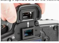
2. Align the groove on the EP-15 with the rails on the camera's viewfinder.
