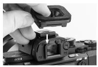
3. Firmly slide the EP-SP down on the viewfinder rails until fully seated.
