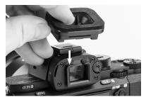
3. Firmly slide the EP-F down on the viewfinder rails until fully seated.
