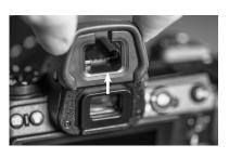
2. Align the groove on the EP-NZ with the rails on the camera's viewfinder.
