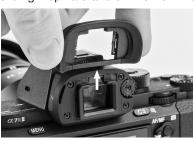
2. Align the groove on the EP-S with the rails on the camera's viewfinder.
