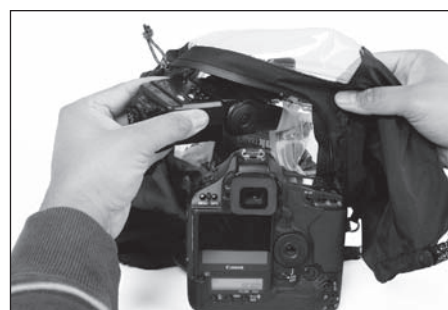
Step 1: Unzip the cover and push the strobe up into the strobe pocket.
