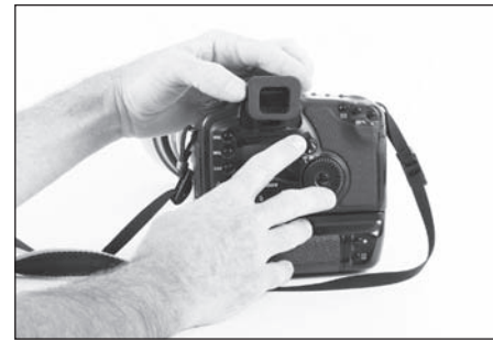
Step 3: Remove the current eyepiece from your camera body and replace it with the correct Think Tank eyepiece.
