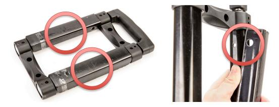
2. Slide the new handle into position on the bag, making sure the holes are correctly aligned as shown. Push all four bolts through the inside bag and into the handle.
