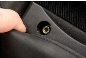
4. Tighten each of the nuts until snug. Use the hex key to hold the bolt in place while you tighten the nut with the socket driver. Do not over tighten the nuts.
