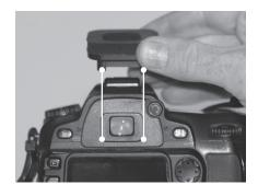
3. Firmly press eyepiece all the way down.
