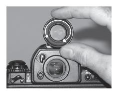
Screw the eyepiece into the camera.
