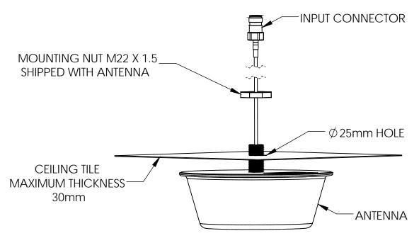
NOTE: SI400 SERIES ANTENNA CAN BE MOUNTED ON METAL OR NONMETAL CEILING.
