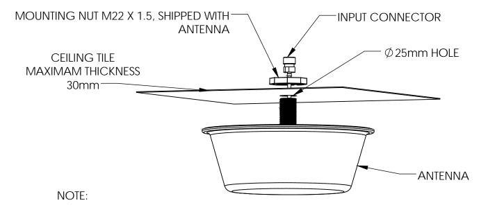
SI300 SERIES ANTENNA CAN BE MOUNTED ON METAL OR NONMETAL CEILING.
