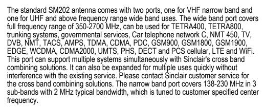
The antenna is fed by two RG303 pigtails with N female connectors. Other connector options are also available.
