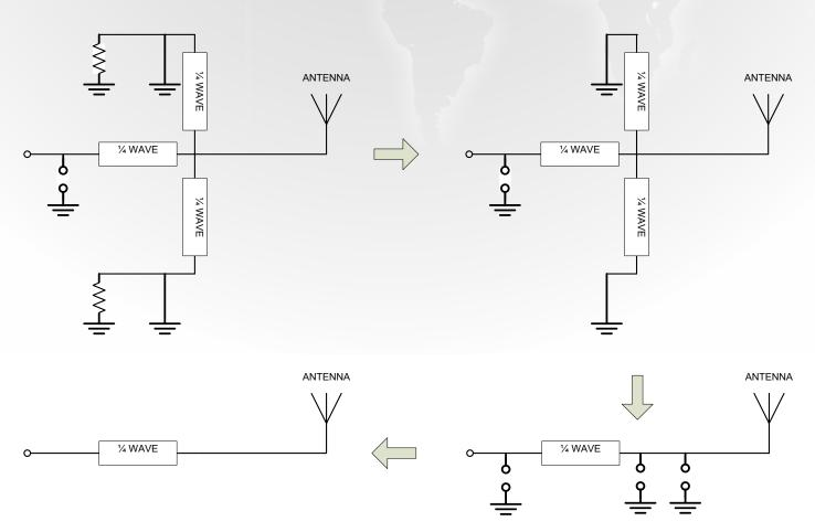
We can see how the rules we have established reduce the circuit to just the antenna and a  $\frac{1}{4}$  wavelength transmission line. If the transmission line is the same impedance as the antenna then the line effectively vanishes and the transmitter only sees the antenna.
