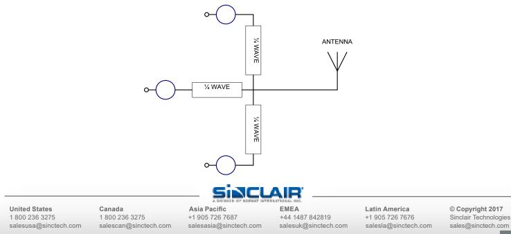
When one cavity is at resonance then the other cavities are off resonance. The approximate circuit is shown below:
