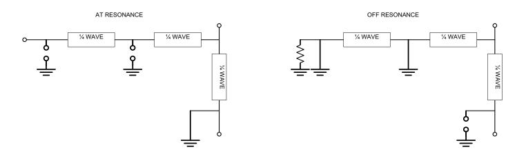
On the next page, we see the equivalent circuit for a combiner made up of three C-series. The center channel is at resonance and the other ones are off resonance. The port near the notch cavity in the last module in the chain is terminated in 50 ohms. Again we see how the rules allow us to reduce the circuit to a length of transmission line going straight to the antenna.
