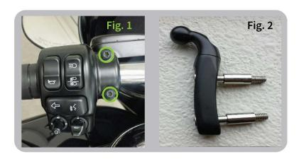
3. Compare the threads of your old bolts to the bolts supplied in the kit. The shorter 1/4-20's are commonly used in newer Harley models. Use the M6 for metric bikes. Prepare the perch mount as shown above. (Fig. 2)
