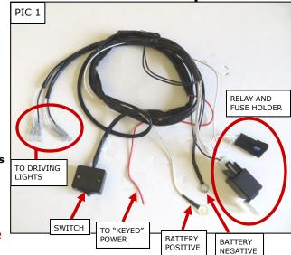
battery before starting this procedure. Avoid potential electrical shock! Disconnect the
