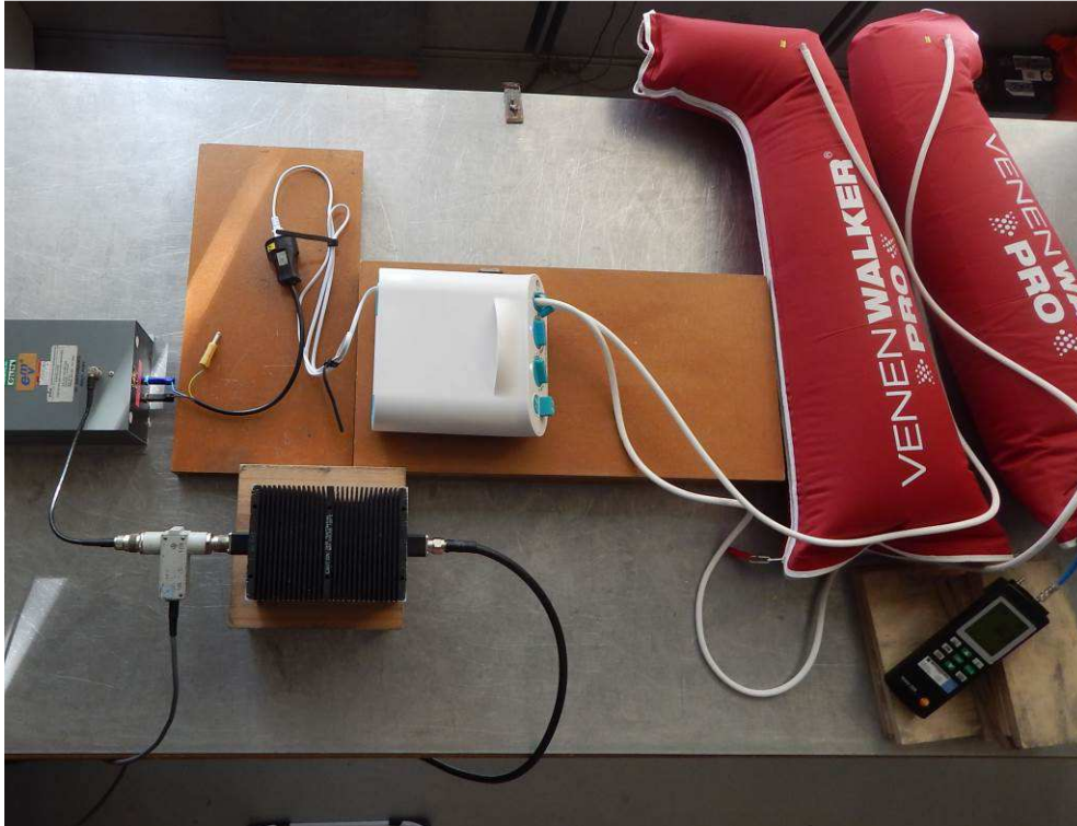
Fig. 9: Test set-up induced by RF fields
