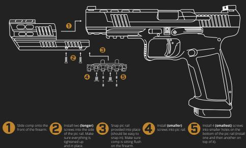
\*The compensator will work without installing the set screws
