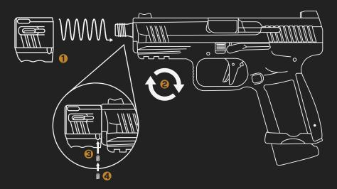
Thread comp onto the muzzle as far as it will go while still staying in line with the slide
