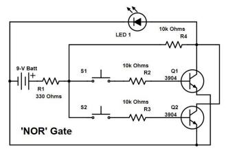
**Explanation of the circuit:** This circuit has two transistors. If you forward-bias either one or both of them the LED will <u>not</u> light up indicating a LO on the output.
