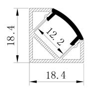
LED Angle 45 Aluminum Channel includes our v-shaped aircraft-grade aluminum channel and compatible frosted or opal white lens. Creating a rigid, modern, and sleek style LED strip light installation has never been easier.
