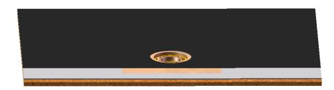
4. Mechanically attach clamping ring with supplied hardware.
