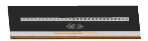
7. Apply morter to desired height. use caution to avoid morter entering weep holes.
