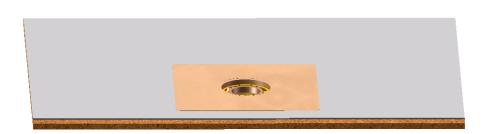
3. Apply waterproofing to drain basin. prime drain flashing if required.
