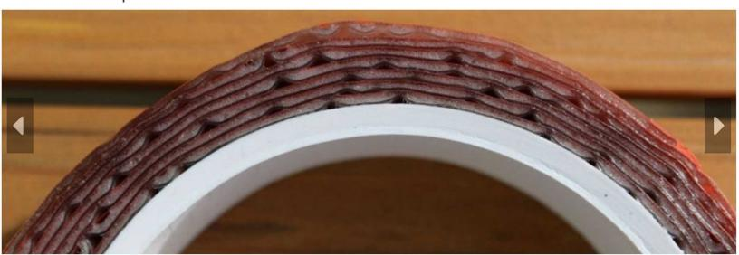
It's also vital that you install the Carogna tape in temperatures ranging from 70-100 degrees Fahrenheit. If you mount in temperatures lower than that, it's possible the tape won't adhere properly. Once the tire and tape are mounted, you'll need to pump up the tires and let them sit for at least eight hours, though Carogna says you'll want to let them sit for 24 hours for full adhesion.
