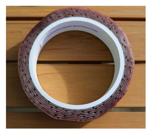
What changed between the first try and the second try? Nothing, except for one step in the process: The first time I mounted the tires, I cleaned the rim with isopropyl alcohol. The tape did not adhere properly. The second time, I used the same alcohol, and once dried, I used Effetto Mariposa's Carogna remover to ensure there was absolutely nothing on the rim that could compromise the tape's application.
