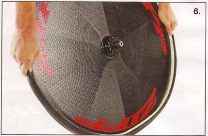
Install the tire on the rim over the top of the pink release tape. Once the tire is on, inflate and shift it to make sure it is aligned straight on the rim.
