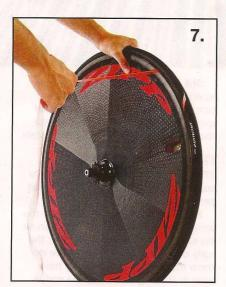
Slowly pull the release tape out from under the tire. Make sure to do this with about 20 PSI in the tire to keep the tape from tearing.
