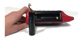
3. Plug in the 2,000 mAh Li-Ion Battery
