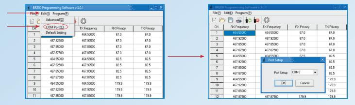
TIP: Most often, your computer will automatically recognize the radio on COM 3. If the data does not successfully transfer using COM3 in Step 9, try a different COM port assignment from the program.
