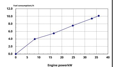
Performance data at atmospheric pressure are100kPa, the intake air temperature is25degrees Celsius, altitude is80m, the water vapor partial pressure is1kPa, use standard0#Under diesel, follow GB/T18297 experimental conditions were obtained.
