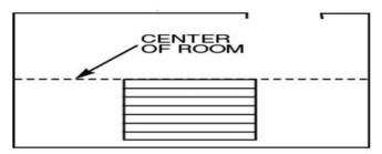
Avoid cutting in pieces less than half the plank width or tile size, if you find the cut in planks or tile will be less, the centre starting line should be moved to allow for minimum half the plank or width. This will "balance" the room and provide for a larger cut piece at the wall.
