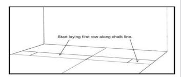
Start by placing a 2 metre straight edge on the floor along the centre line to keep the planks and tiles square.
