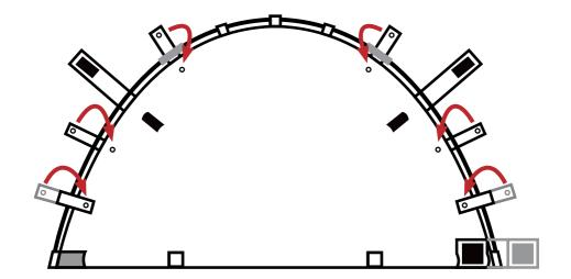
Connect the two lower rods to the main bracket and close the velcro pad.
