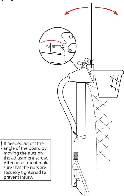
moving the nuts on the adjustment screw. After adjustment make sure that the nuts are securely tightened to prevent injury.
