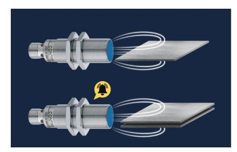
Contrinex smart sensors can utilize the distance measurement principle to determine the presence of one or more sheets in front of the sensor. The configurable detection thresholds of Contrinex smart sensors allow for the detection of various sheet materials and thicknesses using a single sensor.
