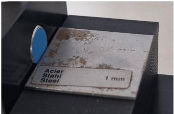
It is also important that the first sheet does not saturate the measurement value beneath 20% to be able to latter on detect an additional sheet.
