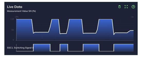
It is shown that the SSC1 switches on only when the predefined level is reached. This indicates that at least on sheet is in position infront of the sensor.
