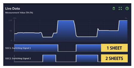
SSC2 will identify excessive target material in front of the sensor, indicating the presence of an extra sheet. The desired threshold can be programmed using any method, causing SSC2 to activate when additional material is detected.
