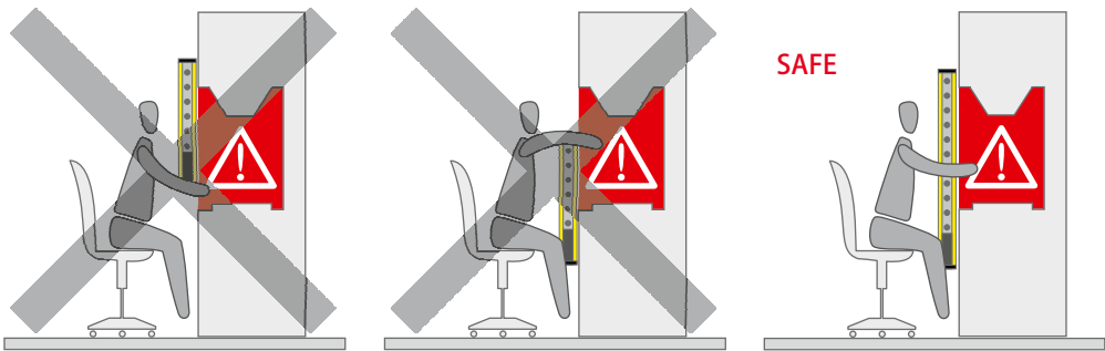
FIG. 4: POSITIONING THE LIGHT CURTAIN
