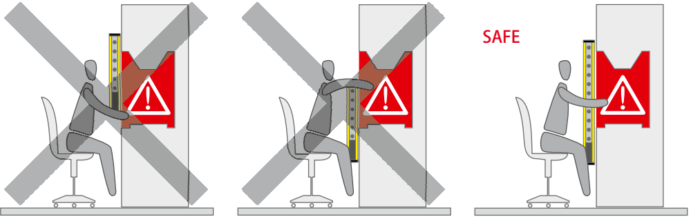
FIG. 9: POSITIONING THE LIGHT CURTAIN
